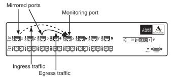
Figure 5-2 Monitoring Ports
